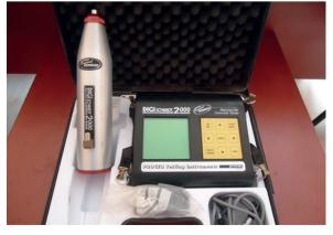
Figure 2. Schmidt hammer hardness test equipment
