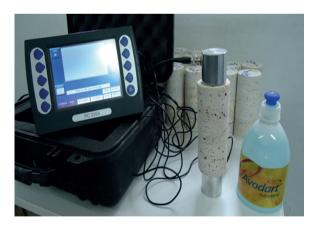
Figure 1. Sound velocity test equipment
